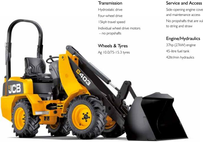
Side-opening engine cover for service and maintenance access
