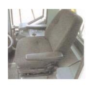
The seat and instrument panel ,are adjustable so that the operator is continually in optimum working conditions - visibility of equipment, user-friendly positioning of controls (Kick-down selection with control switch, steering column adjustment, choice
