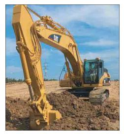
**Tracks.** The 330D comes standard with grease lubricated tracks. The track links are assembled and sealed with grease to decrease internal bushing wear, reduce travel noise and extend service life lowering operating costs.
