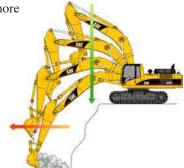
**Truck Loading.** Loading trucks from a bench is more productive and fuel efficient as the return cycle is reduced while the boom down function does not require pump flow.
