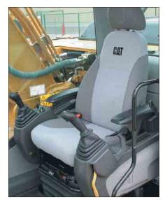
**Consoles.** Redesigned consoles feature a simple, functional design to reduce operator fatigue, ease of switch operation and excellent visibility. Both consoles have attached armrests with height adjustments.
