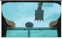
**Skylight.** A unique large polycarbonate skylight provides very good upward visibility, especially useful in above ground applications.
