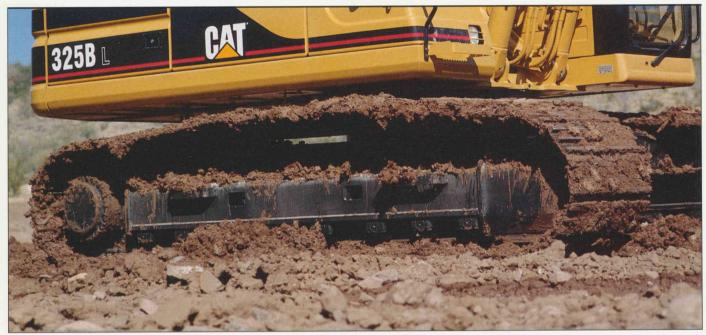
**Precision robotic welding** ensures a quality weld every time. These welds increase rigidity, reduce internal stresses and enhance durability for the chassis and track roller frames.
