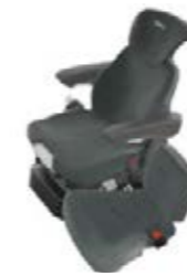
□ The super comfort seat has a seat heater, rotary adapter and pneumatic lumbar support - prerequisites for comfortable work during long shifts.
