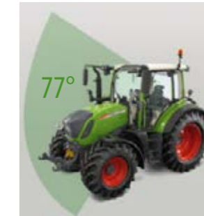
Panoramic windscreen with 77° field of vision for a full view upwards and onto the wheel arches.
