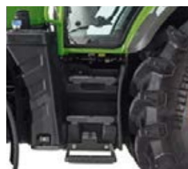
■ Wide step treads permit safe and easy entering and exiting. The door handle is easy to reach from the ground.
