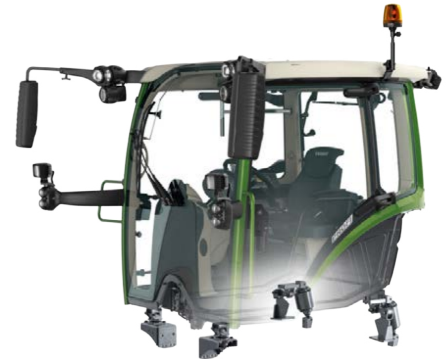
□ The pneumatic cab suspension (Profi and ProfiPlus configuration) reduces vibrations to a minimum and provides high ride comfort. It is supported on four points with integrated self-levelling: the cab rests on two conic bearings at the front and on two air spring elements at the rear.
