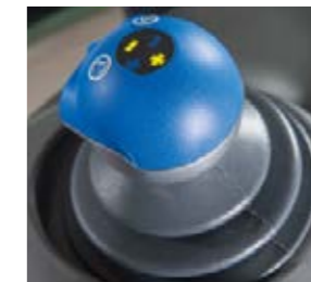
Crossgate lever for 1st and 2nd hydraulic control unit and the front loader, including the controls for the 3rd and 4th circuit.
