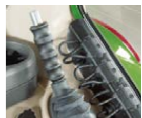
Cables can be led neatly into the cab from the outside through the closed rear window. Dirt and moisture stay outside.
