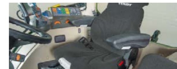
The suspension system and the individual armrest adjustment ensure comfortable work days. The super comfort seat also has seat heating, a rotary adapter and a pneumatic lumbar support.
