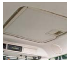
■ The hatch integrated in the roof liner offers additional ventilation on hot days.
