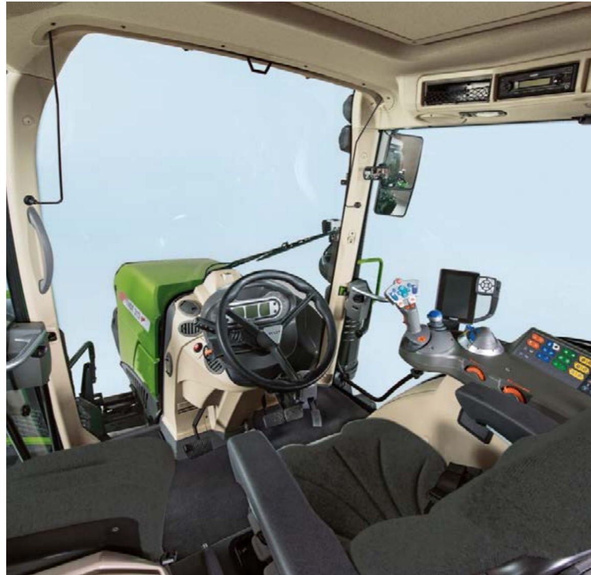
The clearly laid out and ergonomically designed VisioPlus cab offers the best overview, both to the operating elements and the field. The windscreen is available as a continuous panoramic window or as a hinged pane. An additional door can be chosen in place of the right side part.
