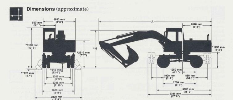
Dimensions shown are for machine equipped with 10.00-20 tires.
