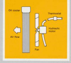
**Hydraulic oil cooler** is independent from engine fan and assures cooling capability in high ambient temperatures. The cooler fan is hydraulically driven and thermostatically controlled for efficiency. A light on the instrument panel indicates when the fan is running at maximum speed.
