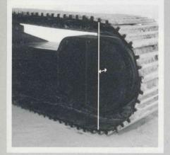
Integrated final drives protect the track motors, disc brakes and hydraulic lines. These components are contained within the envelope of the track shoes, including shoes 19.7"/500 mm wide. Track motor guards are not required.
