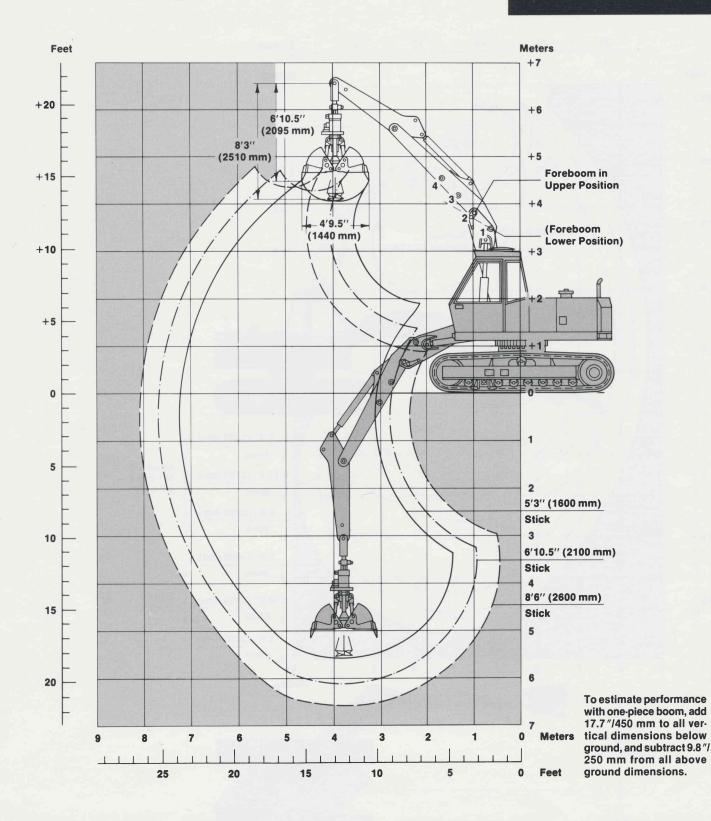
With foreboom in lower position, digging depths are increased 11.6"/295 mm and dumping heights are reduced by:
