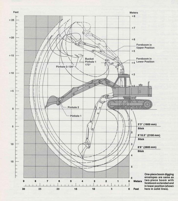
General purpose buckets have two pinholes to adapt bucket to different work conditions. Bucket pinhole #1 provides wide curling arc with less force, and pinhole #2 is for smaller curling arc with more force. Maximum breakout force
