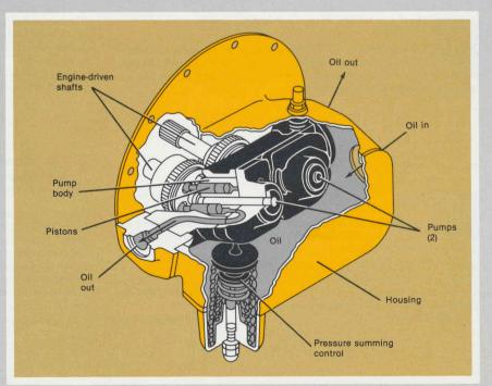
Two variable displacement piston pumps are the key to exceptional productivity. These pumps furnish summated power to the boom, stick and bucket. With summated control, both pumps supply identical flow rates to the system or to a single circuit, as required, for fast implement response and high fuel effiiency. One of the pumps also powers the swing function, and both power the travel circuit.
