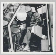
**Left armrest** lifts for operator entry and exit. Raising the armrest prevents actuation of all hydraulic functions except circuits in use at that time.
