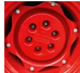
□ Additional wheel weights increase the rear axle traction.
