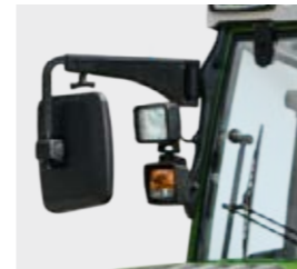
□ On request, the side rear view mirrors can be fitted in a detachable version.
