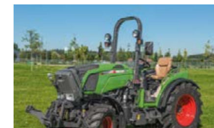
For use in hothouses or in restricted spaces, Fendt offers variants without a roof and with a roll bar.
