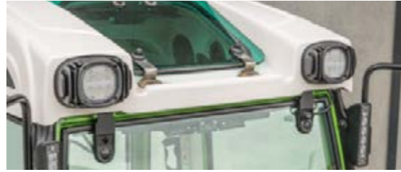
□ Bright LED work lights in the front roof section have a long range.
