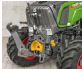
2,540 daN lift capacity is available on the front linkage in the P variant.
