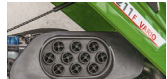
High-performance filter for high separation capacity under difficult conditions.
