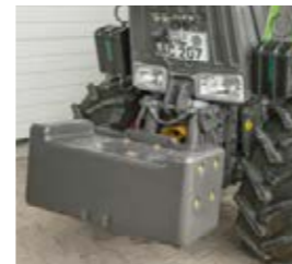
□ The front-end weight provides for a better powertrain function on the front axle.
