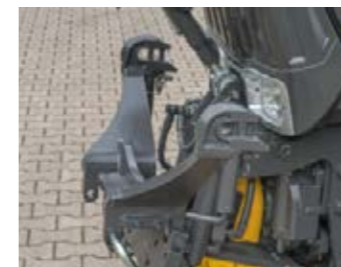
The front hydraulics lower links can be folded compactly in just a few steps.
