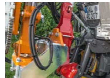
The mounting plates integrated in the front linkage always provide a stable and secure base for heavy front-mounted implements.
