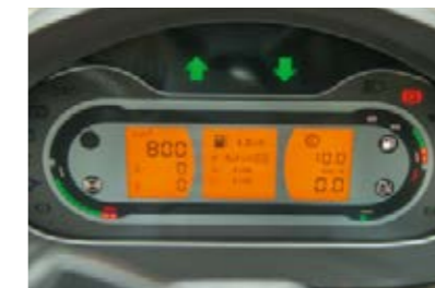
Easy switchover: The multi-function display shows what you need for your work, e.g. the current and average fuel consumption or the worked area.
