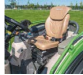
■ The synthetic leather seat is water and dirt-repellent and is a perfect match for models without a roof.
