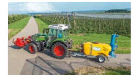
Efficient combination of processes. With the 540E/750 front PTO, you can drive the mulcher at the operating speed, though the sprayer in the rear and the tractor operate at a reduced engine speed.
