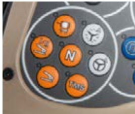
The VarioActive superimposed steering system and the Guidance system can be conveniently activated on the steering wheel console.
