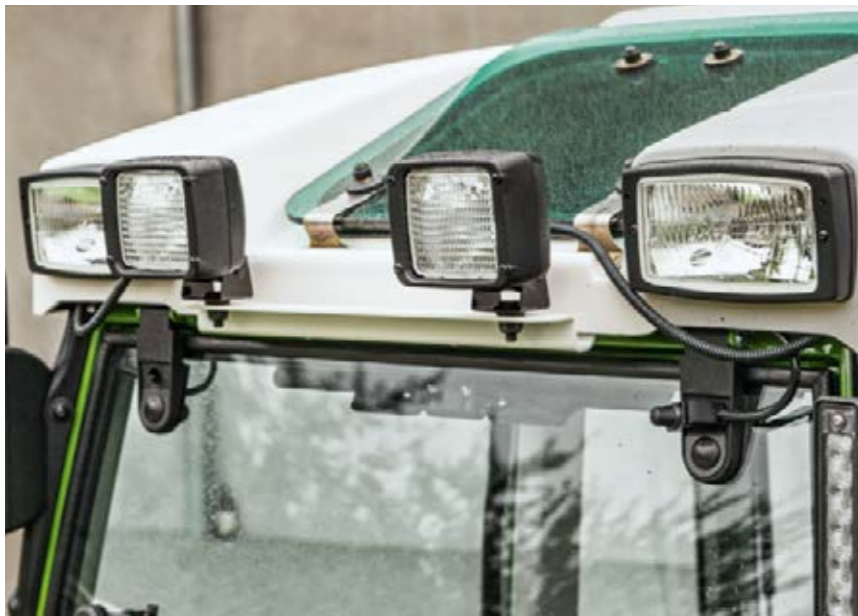
□ Two work lights can also be fitted at the front in the version with auxiliary headlights.
