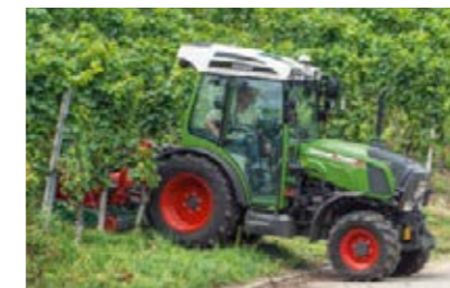
The PTOs operate independent of the road speed. For example, you can drive slowly when mulching a dense uncut crop, and to drive faster, continuously, without changing gears or switching off in sparse crops.
