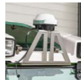
Position-based GPS steering system provide accuracy down to 2 cm in the Fendt 200 V/F/P Vario.
