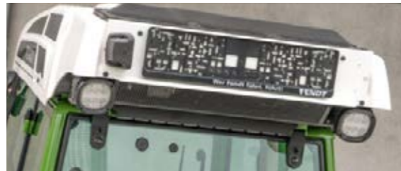
□ Retain an overview of the implements at the back of the roof with the LED work lights.
