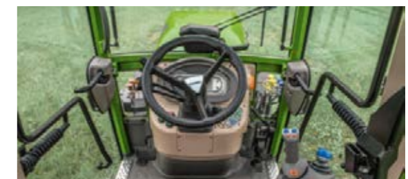
Maintain a good view of your implements with the large glazed area and narrow steering column. For overhead work, e.g. in hops, the roof window provides the ideal view.
