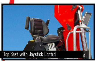
The crane is operated by joysticks in combination with foot levers. The Danfoss PVG 32 control valve with variable flow pump provides a quick and very precise control of movements. The lever sequence is: Left hand: "Slew" and "Jib". Left foot: "Grab". Right hand: "Rotator" and "Boom". Right foot: "Extension".
