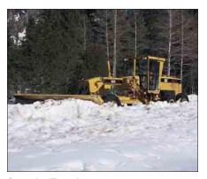
**Superior Traction.** All-wheel drive improves tractive performance in poor underfoot conditions such as snow, mud, and sand. This feature also provides excellent steering and sidedraft control.
