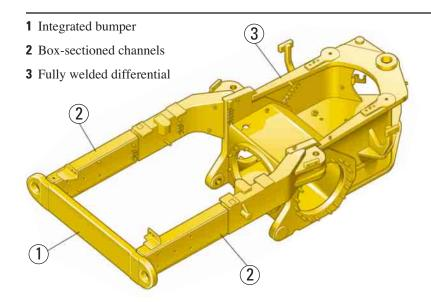
**Integrated Bumper.** The integrated bumper ties the rear frame together into a cohesive unit, to handle the loads possible with the new 3176C power train. This is especially important in ripping and snow removal applications where graders are equipped with snow wing attachments.
