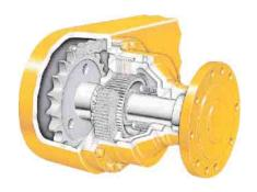
**Brakes.** Caterpillar multi-disc brakes offer a large surface area for dependable, extended-life braking. The air-actuated service brakes, located in each of the four wheel spindle housings, are sealed, adjustment free, and lubricated and cooled by tandem housing oil. The parking/emergency brakes, located in the transmission on the output shaft, are spring actuated and air pressure released. When engaged, they neutralize the transmission and lock the wheels on any surface.
