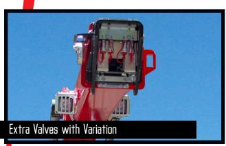
A well-known and usual hose routing to the end of the extensions means that 1 or 2 extra valves are fed in sturdy hose guides alongside the jib extension system. If further efficient protection of the hoses is required, 1 or 2 extra valves can be fed in internal hose reels and lie particularly well protected.
