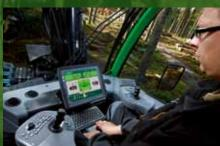
The TimberMatic H-12 is an easy-to-use automation system that both optimizes and facilitates production, timber measurement, and basic machine-control functions. The new PC, HPC14, further helps meet the demanding requirements of the forest industry.
