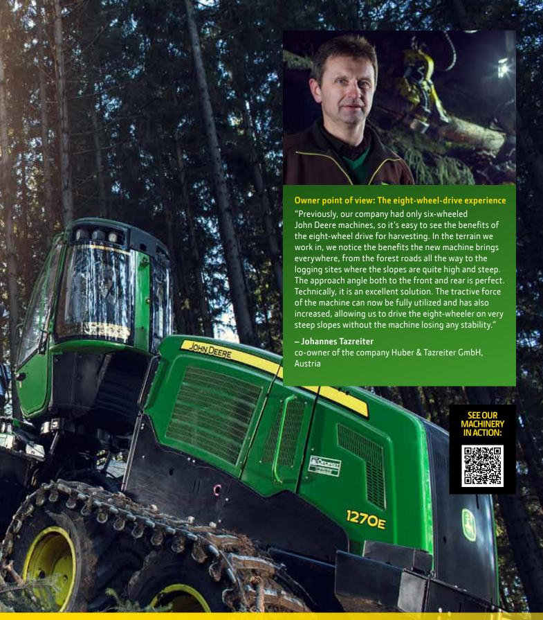
The rotating and leveling cabin turns 160 degrees. Available in both six- and eight-wheel-drive harvester models, it provides 360 deg. visibility to your surroundings and of boom movements, and ensures safe and efficient harvester operation.
