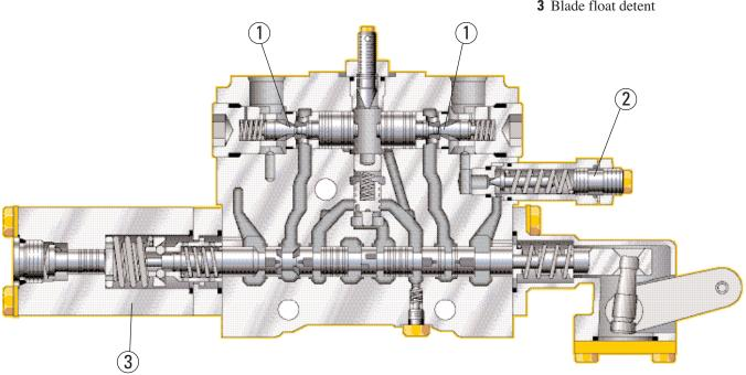
Load Sensing Hydraulics. A load sensing variable displacement pump and the advanced proportional priority pressure-compensating (PPPC, or "triple-PC") hydraulic valves provide superior implement control and enhanced machine performance and efficiency. Continuously matching hydraulic flow and pressure to power demands creates less heat and reduces power consumption.
