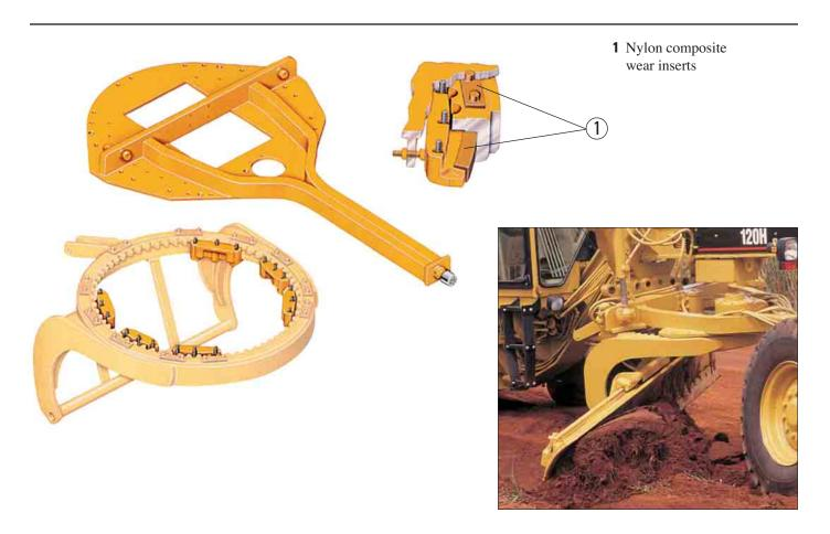
**Blade.** Heat treated moldboard rails, through-hardened, curved DH-2<sup>™</sup> steel cutting edge and end bits, and replaceable metallic wear inserts assure a long, reliable service life. Three sideshift mounting locations for the optional moldboard add flexibility.
