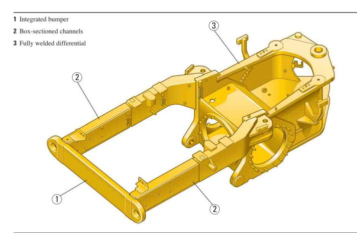
**Integrated Bumper.** The integrated bumper ties the rear frame together into a cohesive unit, to handle the loads possible with the new 3126B power train. This is especially important in ripping and snow removal applications where graders are equipped with snow wing attachments.
