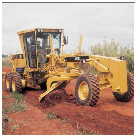
**Quiet Cab.** The resiliently mounted engine and transmission reduce interior engine noise and vibration. Interior sound levels do not exceed 75 dB(A), using ISO 6394. Lower interior noise levels improve operator working conditions.
